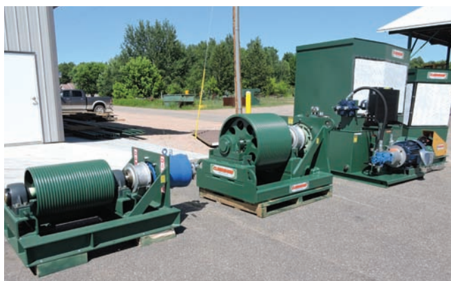
The equipment is as follows, from left to right: 100 HP Hydrostatic Cable Drive, 150 HP Hydrostatic Cable Drive, 50 HP HPU for Cleereman 50 HP Carriage Drive, Custom Sawyers Cab and Standard Sawyers Cab.
